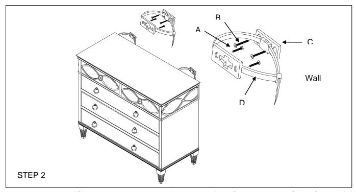
Attach the Brackets (C) horizontally to the top of the back of the Chest using the Small Screws (A). Screw the remaining Brackets (C) vertically 1 inch below the brackets attached to the Chest using the large screws (B). The Large Screws (B) should be screwed into a stud in the wall. Align the Brackets vertically and string in the Retention Belt (D). Confirm Strap is securely laced and locked.
