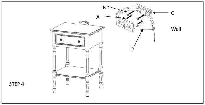
Attach the Brackets (C) horizontally to the top of the back of the Table using the Small Screws (A). Screw the remaining Brackets (C) vertically 1 inch below the brackets attached to the Table using the large screws (B). The Large Screws (B) should be screwed into a stud in the wall. Align the Brackets vertically and string in the Retention Belt (D). Confirm Strap is securely laced and locked.
