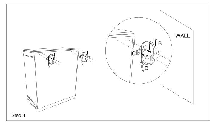
Attach Brackets (C) horizontally to the top of the back of the Cabinet using the Small Screws (A).Screw the remaining Brackets (C) horizontally 1 inch below the brackets attached to the Cabinet using the large screws (B).The Large Screws (B) should be screwed into a stud in the wall. Align the Brackets and string in Retention Belt (D). Confirm Strap is securely laced and locked.
