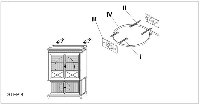
Attach 2 Brackets (III) horizontally to the top corners of the Unit using the Small Screws (I). Screw the remaining Brackets (III) into the wall vertically 1 inch below the previously installed brackets using the Large Screws (II). The Large Screws (II) should be screwed into a stud in the wall. Align the brackets vertically and string in the Retention Belt (IV). Confirm Strap is securely laced and locked.
