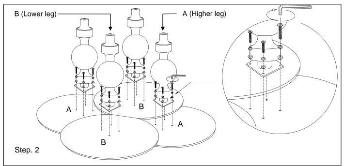
With each corresponding code between legs and top, put the legs aligning the holes of the mounting plate with the female receiving slots of the top. Insert the bolts with its set of lock washer and flat washer then tighten with the Allen key.
