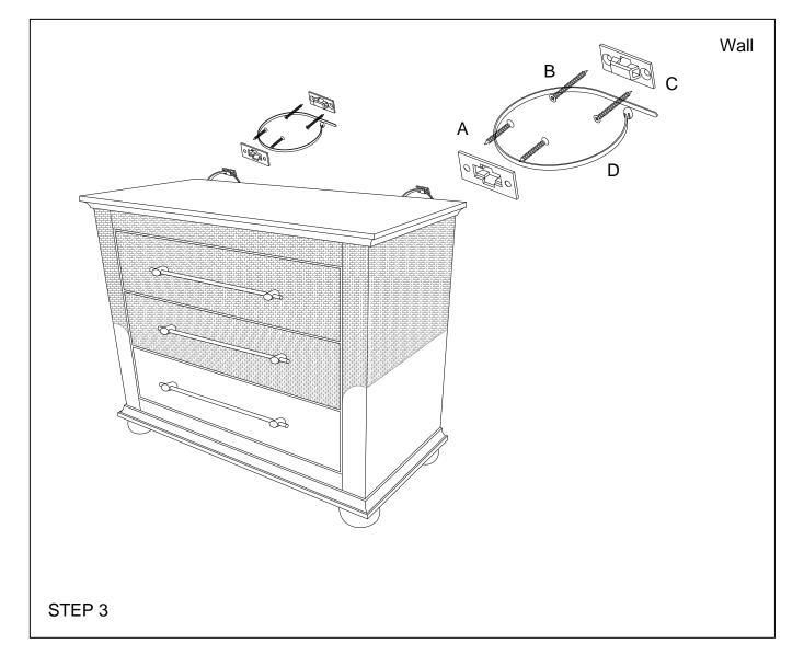
Attach the Brackets (C) horizontally to the top of the back of the Chest using the Small Screws (A).
