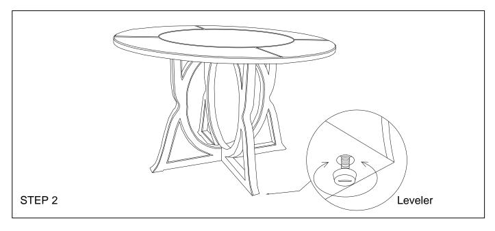
If the floor is uneven adjust the levelers located at the underside of the Leg, to do this lift Up the side that need to be elevated to provide access to the levelers, turn the leveler until adequate contact with the floor.
