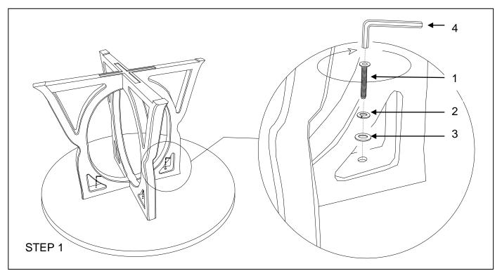
Reverse the assembled pedestal, to attach the PEDESTAL into the pre-drilled holes of the TOP ASSEMBLY, insert the Bolts and tighten with the Allen Key enclosed.
