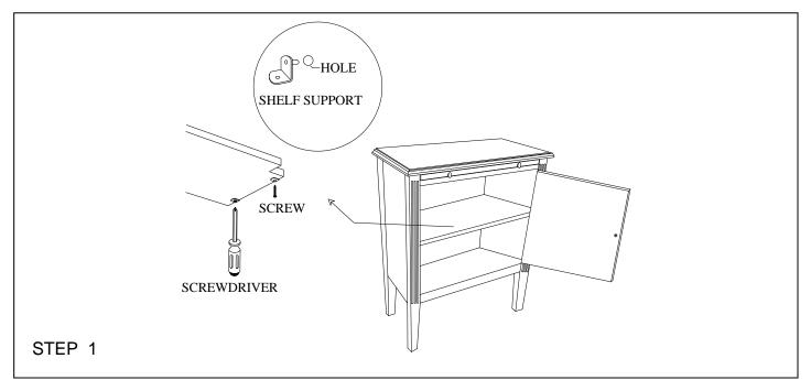
To remove adjustable shelves, remove screw from shelf support, then carefully lift shelves up and out of the case. To reposition adjustable shelves, insert Stem of shelf supports into Holes in End Panel, as shown. Rest the shelf on the shelf supports, and reinstall screws
