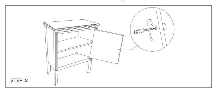
Re-Tighten the bolts from inside of the door using Philip Screwdriver (not included). This can to be done and check periodically to make sure the drawer pull are always tight.
