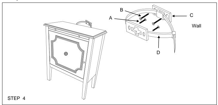
Attach the Brackets (C) horizontally to the top of the back of the Table using the Small Screws (A). Screw the remaining Brackets (C) vertically 1 inch below the brackets attached to the Table using the large screws (B). The Large Screws (B) should be screwed into a stud in the wall. Align the Brackets vertically and string in the Retention Belt (D). Confirm Strap is securely laced and locked.
