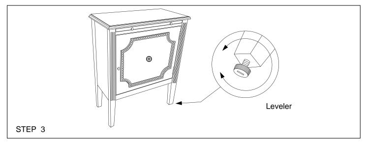
If the floor is uneven adjust the levelers located at the underside of the Leg, to do this lift Up the side that need to be elevated to provide access to the levelers, turn the leveler until adequate contact with the floor.
