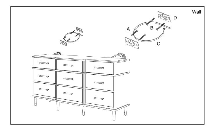
Attach the Brackets (C) horizontally to the top of the back of the Dresser using the Small Screws (A). Screw the remaining Brackets (C) vertically 1 inch below the brackets attached to the Dresser using the large screws (B). The Large Screws (B) should be screwed into a stud in the wall. Align the Brackets vertically and string in the Retention Belt (D). Confirm Strap is securely laced and locked.
