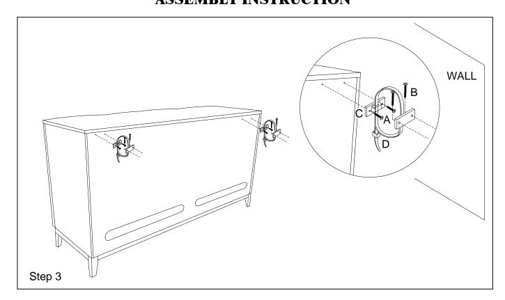
Attach Brackets (C) horizontally to the top of the back of the Cabinet using the Small Screws (A).Screw the remaining Brackets (C) horizontally 1 inch below the brackets attached to the Cabinet using the large screws (B).The Large Screws (B) should be screwed into a stud in the wall. Align the Brackets and string in Retention Belt (D). Confirm Strap is securely laced and locked.
