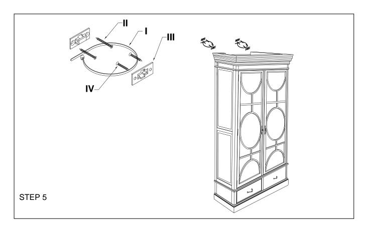
Attach 2 Brackets (III) horizontally to the top corners of the Unit using the Small Screws (I). Screw the remaining Brackets (III) into the wall vertically 1 inch below the previously installed brackets using the Large Screws (II). The Large Screws (II) should be screwed into a stud in the wall. Align the brackets vertically and string in the Retention Belt (IV). Confirm Strap is securely laced and locked.
