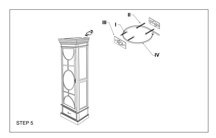
Attach Brackets (III) horizontally to the top corners of the Unit using the Small Screws (I). Screw the remaining Brackets (III) into the wall vertically 1 inch below the previously installed brackets using the Large Screws (II). The Large Screws (II) should be screwed into a stud in the wall. Align the brackets vertically and string in the Retention Belt (IV). Confirm Strap is securely laced and locked.
