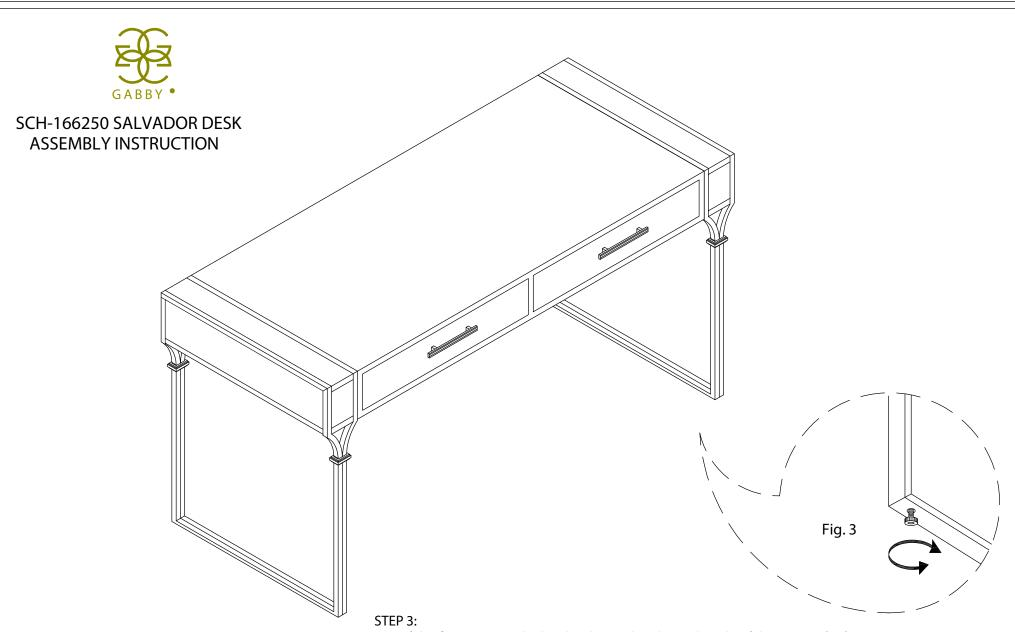
· If the floor uneven the levelers located at the underside of the Leg, to do this lift Up the side that need to be elevated to provide access to the levelers, turn the leveler until adequate contact with the floor as shown Fig.3
