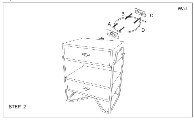
Attach the Brackets (C) horizontally to the top of the back of the Nightstand using the Small Screws (A). Screw the remaining Brackets (C) vertically 1 inch below the brackets attached to the Desk using the large screws (B). The Large Screws (B) should be screwed into a stud in the wall. Align the Brackets vertically and string in the Retention Belt (D). Confirm Strap is securely laced and locked.
