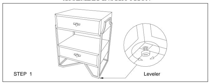
If the floor is uneven adjust the levelers located at the underside of the Leg, to do this lift Up
