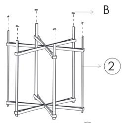
Step 2: Plase 6pcs glass pad (A) on the base (2). Then put the glass top (1) on the glass pad carefully.
