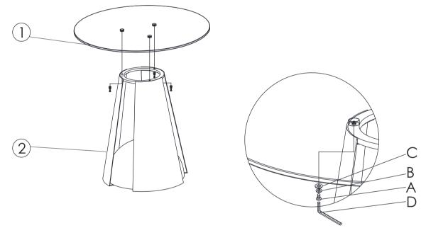
Step 3: Insert 3 pcs Hex Head Bolt(A) through the Lock Washer(B), Flat Washer(C) into 3 holes, fasten with Hex Wrench(D) .
