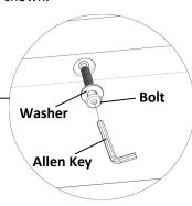
\*secure one side first with bolts and tighten them with Allen keys provide.
