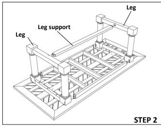
2 person needed to assemble. Place TOP on flat floor , place leg mortise holes to apron tenons & leg support tenons.
