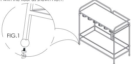
Step 2: The Fisher (E) (wall insert) should be used in conjunction with using a wall stud as anchor. The combination will make the unit very stable. Screw the remaining Bracket (C) vertically approximately 1 inch below the Bracket attached to the console table using the Long Screws (B). The Long Screws (B) should be screwed into a stud in the wall. The Retention Belt (D) go through back metal bar of the console table and the bracket (C) on the wall, then lock it.
