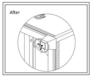
For Anti-Tip Kit: Attach the brackets (C) horizontally to the back of the chest using the small screws (A). Screw the remaining brackets (E) vertically 1 inch below the brackets attached to the chest using the large screws (B). The large screws (B) should be screwed into a stud in the wall. Align the brackets vertically and string in the retention belt (D). Confirm strap is securely laced and locked.
